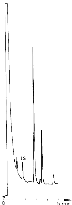
Fig. 4. Gas chromatogram of an extract from 5 ml of pure urine. IS = internal standard (N-methylphthalimide).
